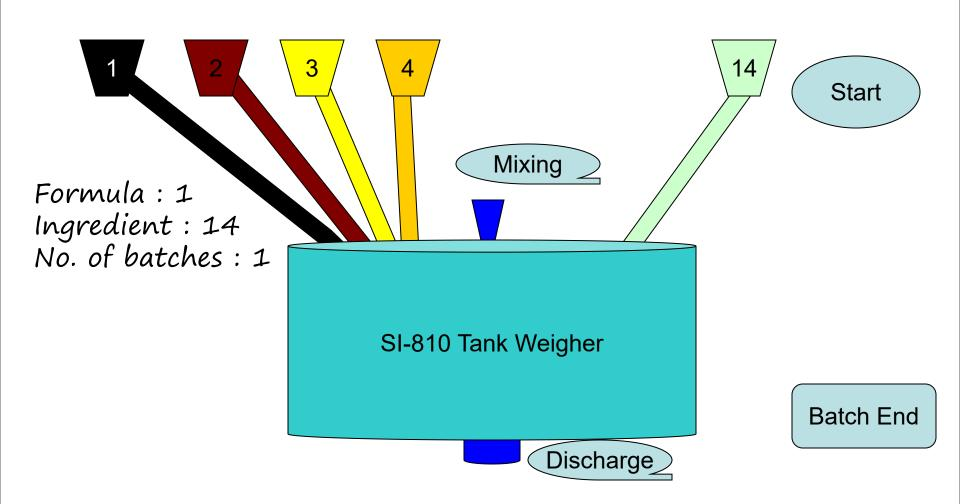
Maximum 14 Ingredients can be controlled through Digital I/O
